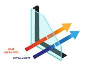
Untreated glass allows heat and UV rays to pass through.
